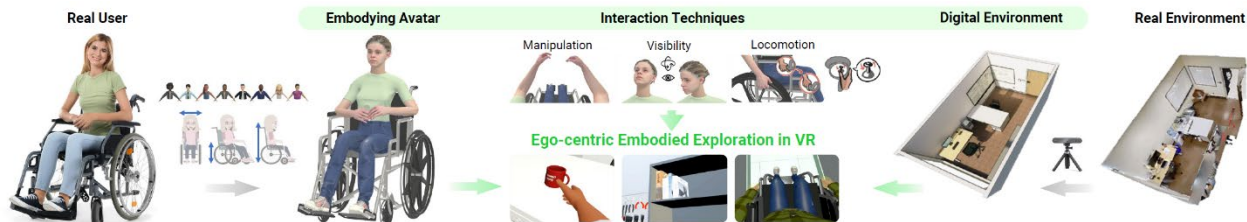
Figure 6: Embodied Exploration consists of three components – a digital environment, an embodying avatar, and interaction techniques. The user is embodied by an avatar, which is generated with biometric information about users and their specific wheelchair model.
