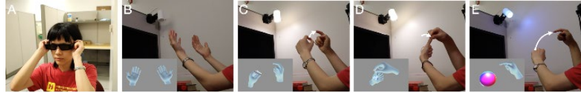
Figure 3: Hand Interfaces allows users to quickly control a smart lighting system by retrieving a digital toggle switch, a joystick for orientation, and a spherical color picker. The user can easily dismiss the tools by taking hands back.
